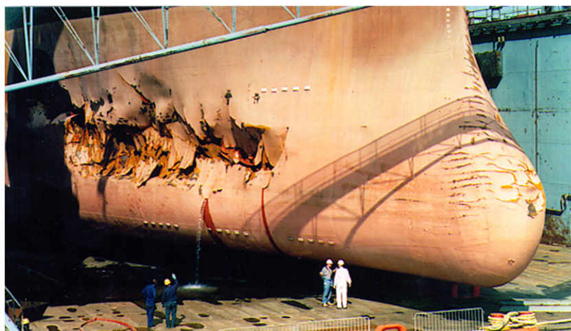
Fig. 9. Image showing damage to the bulk carrier Reduta Ordonia resulting from a sliding-type ice collision below the waterline. The prominent gouging-type rupture is similar to that which occurred in the present simulation. (Photo credit: Andrew Kendrick).
