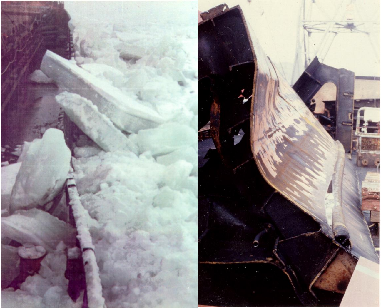
Fig. 24. A ship stuck in compressive ice and the damages that resulted from the compressive ice.
