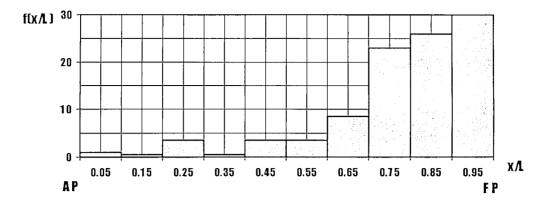
Fig.3.1. Distribution density of nondimensional longitudinal damage location
