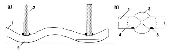
Fig.2.2. Wear of plates of the shell plating of icebreakers
