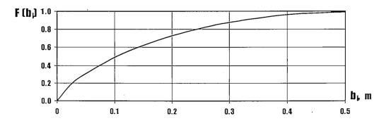
Fig.3.4. Distribution function of transverse damage penetration
