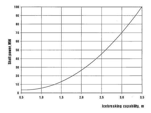
Fig.4.1. Dependency of the shaft power on the icebreaking capability of modern icebreakers with the improved conventional hull shape
