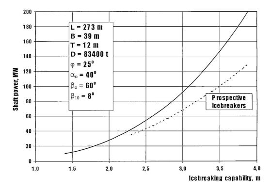
Fig. 5.1. Relationship between power and icebreaking capability of a large arctic containership with a capacity of 3000 TEU with the improved traditional hull lines shape and the triple-shaft propelling unit
