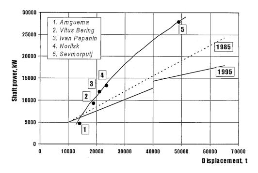
Fig.4.7. Minimum shaft power of ULA category ships according to 1985 and 1995 requirements
