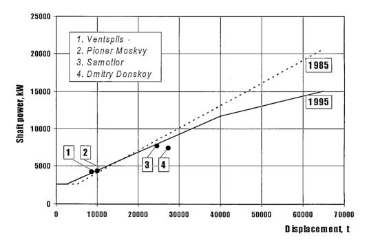
Fig.4.8. Minimum shaft power of UL category ships according to 1985 and 1995 requirements
