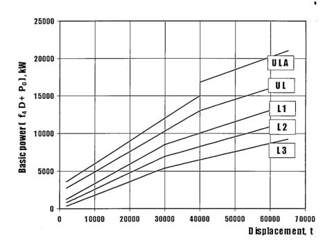
Fig.4.4. Dependence of the basic power of ships of different ice categories upon the displacement
