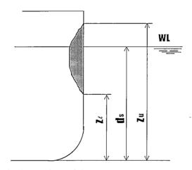
Fig.3.5. Vertical location of damage
