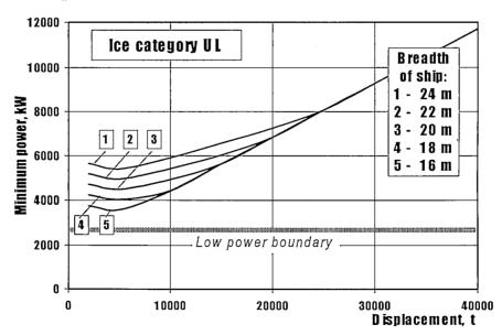
Fig.4.6. Minimum shaft power according to the MRS requirements for ships of UL category (with FPP) depending on the displacement and breadth
