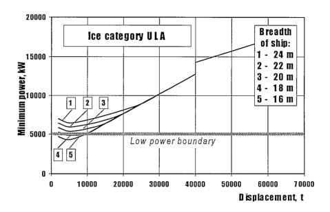
Fig.4.5. Minimum shaft power according to the MRS requirements for ships of ULA category (with CPP or FPP) depending on the displacement and breadth
