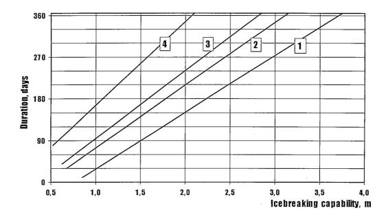
Fig. 5.2. Relationship between duration of the safe independent navigation of traditional icebreaking cargo ships in the Arctic and the icebreaking capability (taking into account the long-standing experience of carrying out arctic operations): 1 — eastern area of the Arctic and transit navigation along the NSR, 2 — western area of the Arctic, 3 — western part of the Kara Sea, 4 — Pechora Sea
