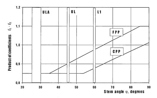
Fig.4.2. Influence of the stem angle on the product of coefficients  $\mathbf{f_1} \cdot \mathbf{f_2}$  with due account of the type of propulsion plant
