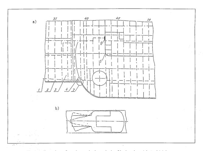
Fig.2.1. Location of cracks on the boat deck of icebreaker *Admiral Makarov* produced during the winter sailing in the Sea of Okhotsk in December 1979 (a); deck swinging pattern (b)
