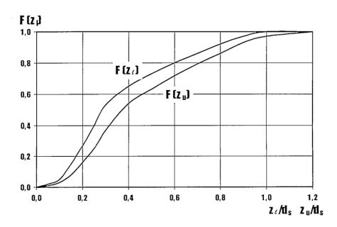
Fig.3.6. Distribution functions of nondimensional vertical damage location
