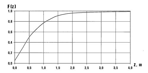
Fig.3.7. Distribution function of vertical damage extent
