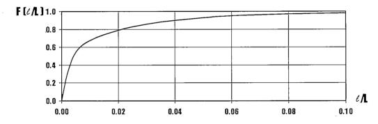
Fig.3.3. Distribution function of nondimensional longitudinal damage extent
