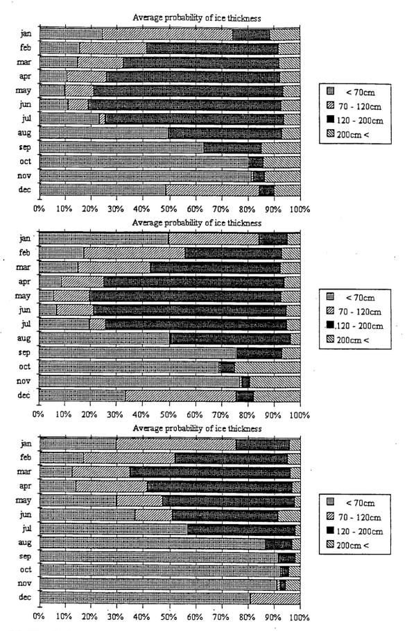
Figure 5.2 Distribution of ice thicknesses along the coastal route during multi-year (top), in 1983 (middle) and in 1990 (bottom).
